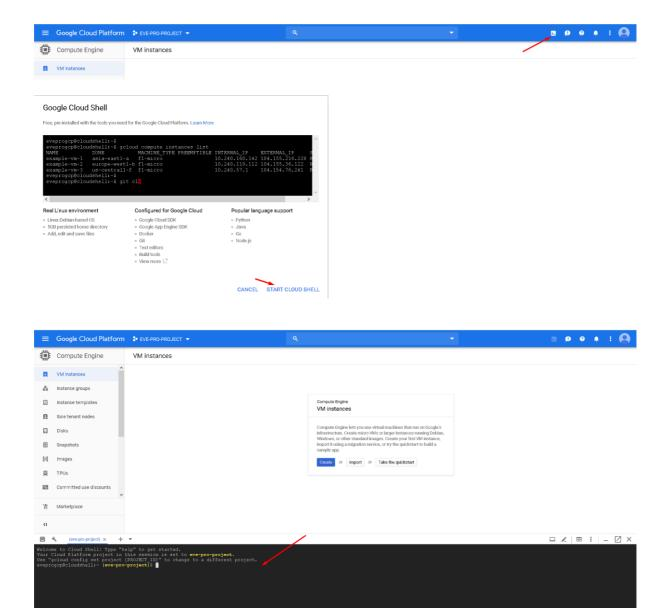
Step 2: create a nested Ubuntu 16.04 image model. Copy and paste the below command into the shell. Use copy/paste. crtl +c/ctrl +v. It is single line command (copy all command below in cli). Confirm with "enter":
