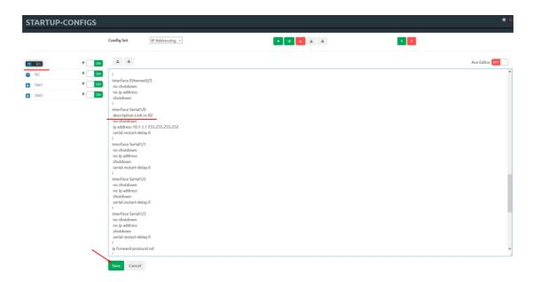
Step 3: Apply the config set to all nodes with the green "Apply Config Set" button on the right (Set all nodes to selected config set).
