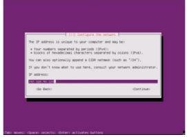
Step 9: Correct your subnet mask, using the Tab key select "Continue" and confirm with Enter
