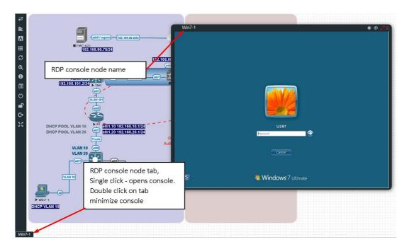
▲ IMPORTANT NOTE: For all Windows nodes, the console type must be set to RDP-TLS in the node template. RDP-TLS node console option is actually only used with HTML5 RDP sessions.
