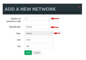
Step 3: Connect your lab node to Private cloud. Your connected nodes in Lab1 and Lab2 will work like being connected to the same network. CDP works. It is convenient if it is necessary to have connections across the multi labs.
