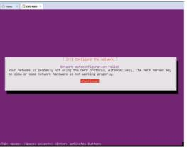
Step 7: Confirm selection "Configure network manually" with Enter
