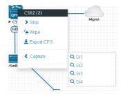
**Capture**. Integrated live Wireshark capture. Select the interface which you wish to capture. Reference section 12
