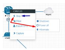
**Stop.** Blue arrow: clicking on Stop will stop the node depending on the method the node supports (power off / shutdown are auto-selected based on the template)
