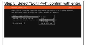
Step 6: Hit Enter, to select IPv4 method. Use down arrow key to select Manual. Confirm with Enter
