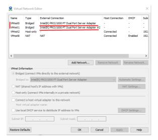
EVE VM Settings. Network adapter is bridged to VMnet0 (ethernet Intel Pro 1), and Network adapter 2 is bridged to VMnet1 (ethernet Intel Pro 2).
