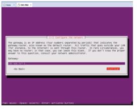
Step 11: IMPORTANT. The name server must be able to resolve public DNS entries and will be used during the next install steps. Enter your name server IP, using the Tab key select "Continue" and confirm with Enter
