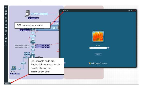
IMPORTANT NOTE: For all Windows nodes, the console type must be set to RDP-TLS in the node template. RDP-TLS node console option is actually only used with HTML5 RDP sessions.
