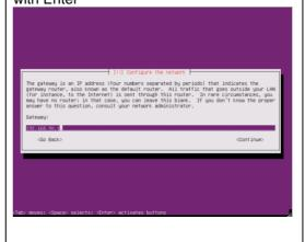
Step 11: IMPORTANT. Name server must respond to the Internet and will be used during the next install steps. Enter your name server IP. Using the Tab key select "Continue" and confirm with Enter
