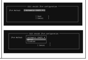
Step 7: Using Tab key fill your network settings. Select Save and confirm with Enter. The name server must be able to resolve public DNS entries!
