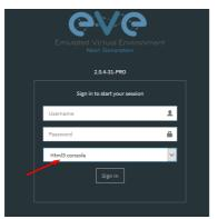
The EVE PRO HTML5 console provides a clientless solution for managing labs and node sessions. Management is achieved directly through the browser by using the Apache Guacamole HTML5 Engine. It is very convenient for Corporate users with restricted Workstation permissions (Locked Telnet, vnc, rdp).
