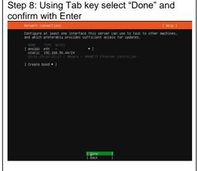
Step 9: Select Done and confirm with Enter. If required, proxy settings can be configured later using EVE WEB GUI System/System Settings described in section 3.5.3
