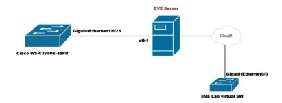
The EVE lab switch's CDP neighbor is the 3750E switch's port Gig 1/0/25: A trunk has been configured between the EVE lab switch and the physical 3750E switch.
