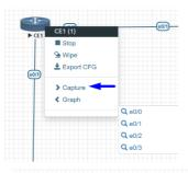
**Capture**. Integrated live Wireshark capture. Select the interface which you wish to capture. Reference section 12
