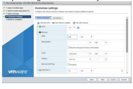
Step 7: Set the size of HDD for your new EVE VM. It is recommended to set "Thick Provisioned eagerly provisioned". Server EVE HDD is recommended to set at least 500Gb
