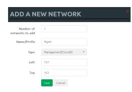
Step 1: Add A New Network onto the topology. There are two ways to do this: Right-clicking on topology area and selecting "Network" or in the sidebar, "Add an Object" and then select "Network."
