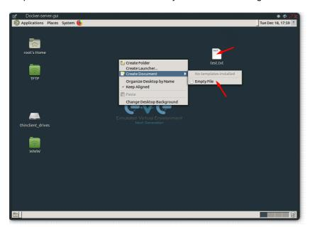
Step 2: Navigate to the desktop of the HTML5 server-gui station and double click **thinclient\_drives** and navigate to: **thinclient\_drives/GUACFS/Download/**
