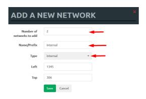
Step 2: Connect your lab nodes to internal cloud. Your configured nodes will work like being connected to the same switch (or the same bridge in EVE). CDP works. It is convenient if it is necessary to have connections across the lab and you don't want to have connections going from one end of the lab to the other.
