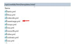
Step 3: Make a copy from source template newimage.yml. Example: Using CLI create template and name it ngips.yml.
