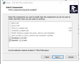
NOTE: The Wireshark option for EVE Professional is left unchecked, because Wireshark is already integrated into EVE PRO.
