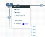
**Graph**. Integrated live interface activity monitoring. Displaying live interface utilization activity.
