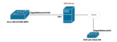
The EVE lab switch's CDP neighbour is the 3750E switch's port Gig 1/0/25: A trunk has been configured between the EVE lab switch and the physical 3750E switch.
