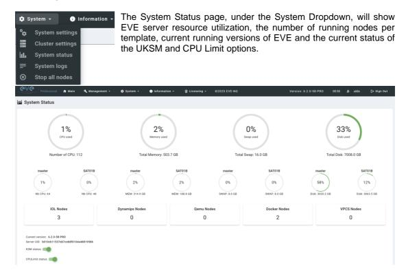
KSM – "KSM (kernel same-page merging) is a Linux kernel feature that allows the KVM hypervisor to share identical memory pages among different process or virtual machines on the same server." It can be disabled globally for EVE on this page. It is recommended to keep KSM **enabled**.
