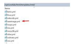
Step 3: Make a copy from source template newimage.yml. Example: Using CLI create template and name it ngips.yml.
