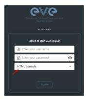
The EVE PRO HTML5 console provides a clientless solution for managing labs and node sessions. Management is achieved directly through the browser by using the Apache Guacamole HTML5 Engine. It is very convenient for Corporate users with restricted Workstation permissions (Locked Telnet, vnc, rdp).
