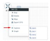
**Capture**. Integrated live Wireshark capture. Select the interface which you wish to capture. Reference section 11
