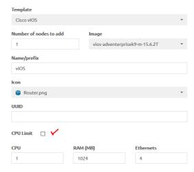
CPU Limit – CPU limit is used to limit CPU overloads during the nodes run time. It acts like a smart CPU usage option. If a running node reaches 80% CPU utilization, the CPU Limit feature throttles CPU use for this node to 50% until process usage drops under 30% for a period of 1 minute.
