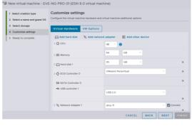
Step 7: Set the size of HDD for your new EVE VM. It is recommended to set "Thick Provisioned eagerly provisioned". Server
