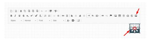
Step 4. Use link button to assign custom protocol for your object. Example: Protocol Other, type in URL: **telnet://10.1.1.10**
