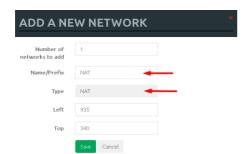
Step 1: Add A New Network onto the topology. There are two ways to do this: Right-clicking on topology area and selecting "Network" or in the sidebar, "Add an Object" and then select "Network."
