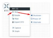
**Stop.** Blue arrow: clicking on Stop will stop the node depending on the method the node supports (power off / shutdown are auto-selected based on the template)
