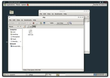
Step 4: Open the destination node's (R1) console and use the tftp command to copy your file:
