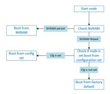
**NVRAM**: NVRAM is used as writable permanent storage for the startup configuration. During the boot process, the node will always check NVRAM for a saved configuration. Saving the configuration to NVRAM requires a vendor specific command. Cisco: copy run startup (wr), Juniper: commit, etc. It is MANDATORY to save a node's configuration before you can export it.
