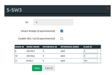
VLAN ID 0 – untagged port with native VLAN 1, used for trunk assignment.
