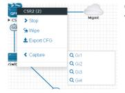
**Capture**. Integrated live Wireshark capture. Select the interface which you wish to capture. Reference section 12
