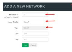
Step 2: Connect your lab nodes to Cloud7. Your configured nodes will work like being connected to the same switch (or the same bridge in EVE). Even CDP works. It is convenient if it is necessary to have connections across the lab and you don't want to have connections going from one end of the lab to the other.
