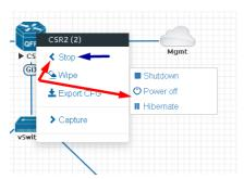
**Stop.** Blue arrow: clicking on Stop will stop the node depending on the method the node supports (power off / shutdown are auto-selected based on the template)
