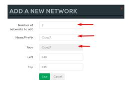
Step 2: Connect your lab nodes to Cloud7. Your configured nodes will work like being connected to the same switch (or the same bridge in EVE). Even CDP works. It is convenient if it is necessary to have connections across the lab and you don't want to have connections going from one end of the lab to the other.
