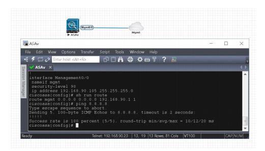
**NOTE:** Cloud interfaces can be used to connect multiple nodes to a single cloud instance on the topology.
