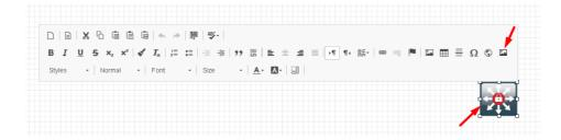
Step 4. Use link button to assign custom protocol for your object. Example: Protocol Other, type in URL: telnet://10.1.1.10
