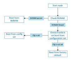
NVRAM: NVRAM is used as writable permanent storage for the startup configuration. During the boot process, the node will always check NVRAM for a saved configuration. Saving the configuration to NVRAM requires a vendor specific command. Cisco: copy run startup (wr),
