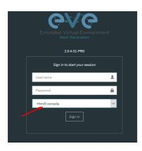
The EVE PRO HTML5 console provides a clientless solution for managing labs and node sessions. Management is achieved directly through the browser by using the Apache Guacamole HTML5 Engine. It is very convenient for Corporate users with restricted Workstation permissions (Locked Telnet, vnc, rdp).
